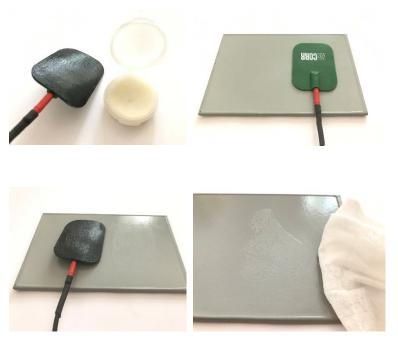
The paste electrolyte forms a purely ohmic contact between the electrode surface and the coating, therefore not interfering with the coating impedance measurement. For details of the electrolyte composition, its electrochemical characteristics and MSDS, please see the ReCorr® QCQ Paste Electrolyte documents provided with the device or contact us at info@recorrtech.com.
