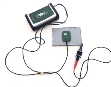
Figure 2. ReCorr® QCQ one-electrode setup.
