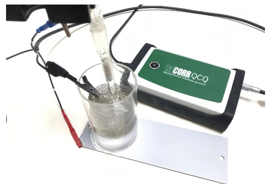
Figure 3. Glass cell three-electrode setup.
