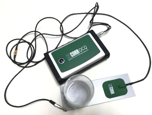
Figure 2. ReCorr® QCQ one-electrode setup.
