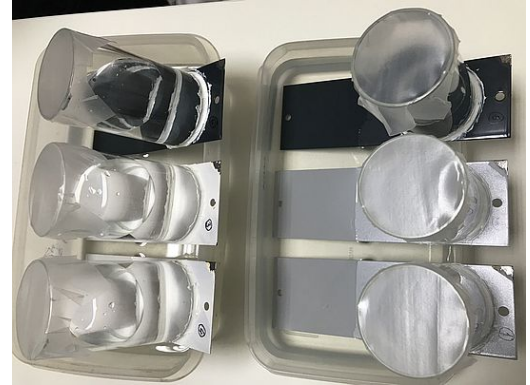
Figure 1. Sample exposure to 3.5% NaCl.
