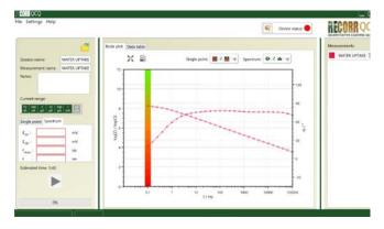
**Barrier coatings with absorbed water** show a fall in *log(Z)* and a decrease in the *phase angle* at low frequencies.
