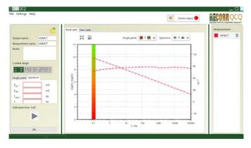
**Intact or excellent** barrier coatings show almost linear log(Z) and a *phase angle* close to -90° in the whole frequency range.
