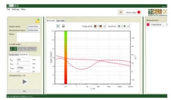
**Coatings with corrosion at the substrate** show a plateau of the log(Z) at medium frequencies followed by further increase in log(Z). The *phase angle curve* first falls then raises attaining a maximum at low frequencies.
