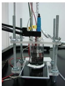
Electrochemical cell for EIS measurements.
