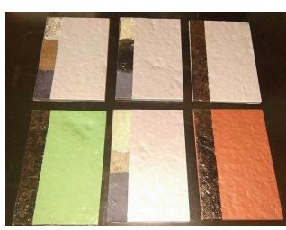
Specimens with rust converters and polymer coatings applied to surfaces prepared by different cleaning methods.
