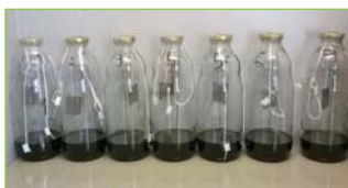
Experimental setup for the mass loss measurements. In each bottle, a coupon was laid at the bottom, with its upper side exposed to the liquid, and its bottom side isolated with tape. Also, in each bottle, one coupon was suspended above crude oil.
