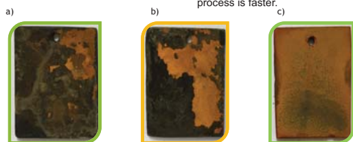
Appearance of the rust layer after 30 days of exposure to: a) inhibitor free solution, b) 60 ppm of VCI 629 BIO in 3.5% NaCl and c) 2000 ppm of VCI 629 BIO in 3.5% NaCl. Black layer presents magnetite and brown-orange lepidocrocite.
